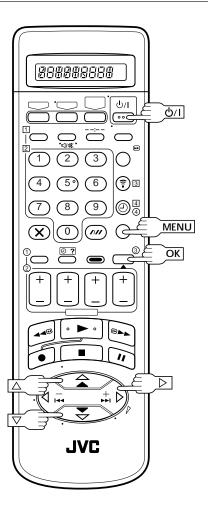
This recorder offers you the choice to view on-screen messages in 10 different languages. Though Auto Set Up selects the language automatically ( pg. 9), you can change the language setting manually using this procedure as required.
